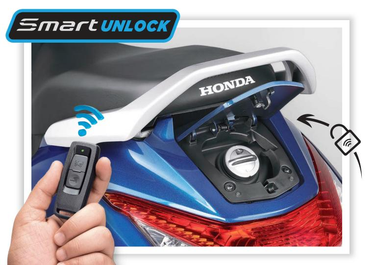
Your two-wheeler key isn't always handy, but with Honda Smart Key, you won't need the key in hand. When the Smart Key is within the **2 meter range** of Activa, you push and rotate the knob to perform various operation like your **seat, fuel cap and handle** can all be unlocked just like that.
